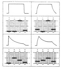
\*\* When all of the ADSR sliders are set to zero, the waveform will be an extremely short Pulse wave, and only a short "click" is heard. Please be careful.
