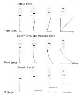
\* In the figure shown above, the positions of the knob are not meant to be exactly correct, so the knob position does not necessarily correspond with the time and the voltage. · Setting of ADSR and Envelope Curve.
